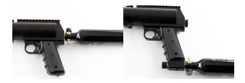
A bottom line ASA can easily be installed by using a 5/64 Allen key to remove the (2) 8-32 button head screws at the bottom of the launcher. Then use a 9/64 Allen key to install the long 8-32 socket cap screws and ASA.
